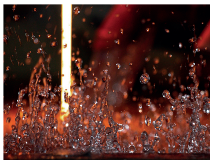
Frit is melted at 1450 °C
