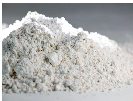
Zirconium silicate gives glaze its white colour
